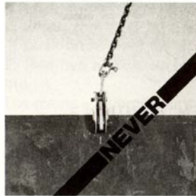
Photograph E (Typical) Excessive side-loading.
