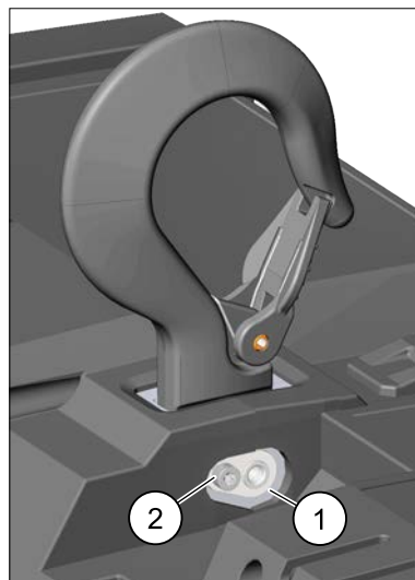
Figure 5. Suspension Pin Retainer/Retainer Screw
