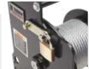
A load holding lock-out pin secures the drum to the frame for secondary load holding and to prevent unauthorized use.
