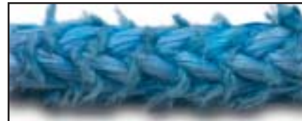
FIG. 3 Severely abraded rope
