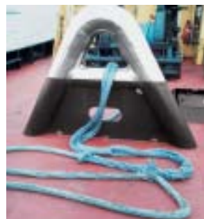
Strop to main line connection.
